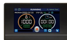
4.3" Touch Screen Data Storage, Data Export to USB Flash Drive (Optional)
